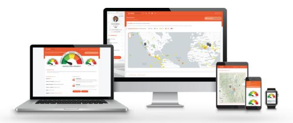
The dashboard includes advanced features such as sensor display, a map of most recent earthquakes around the globe, fault maps, etc. It also provides an asset management layout showing all relevant structural, geotechnical, seismic hazard and other information relevant to the monitored structure.
